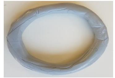
**SPITA ResQ-tape Putty** is a silicone putty for use in cracks and voids in damaged pipes or hoses. The putty molds easily into small cracks or pinholes on pipes and rigid hoses. Excellent for sealing air and steam leaks in combination with SPITA ResQ-tape. The putty always needs to be overwrapped with SPITA ResQ-tape to keep it in place.
